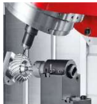
Figure 6. Grinding process with finger abrasive stone on RDB milling machines
