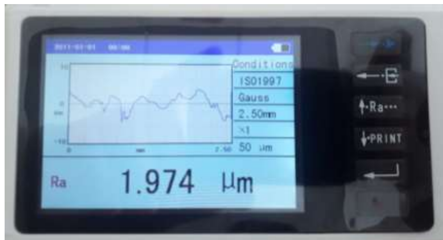
Figure 7. Measurement of R_a using TIME 3221 digital profilometer
