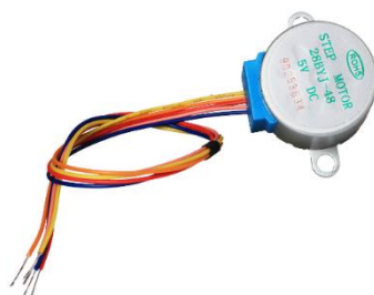
1-rasm. 28byj-48 markali qadamli dvigitelning ko'rinishi
