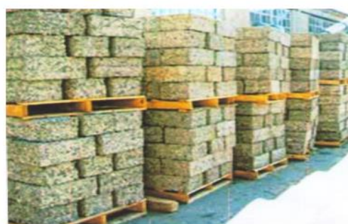
Figure 2. Maturation of arbolite blocks in natural conditions in a warehouse
